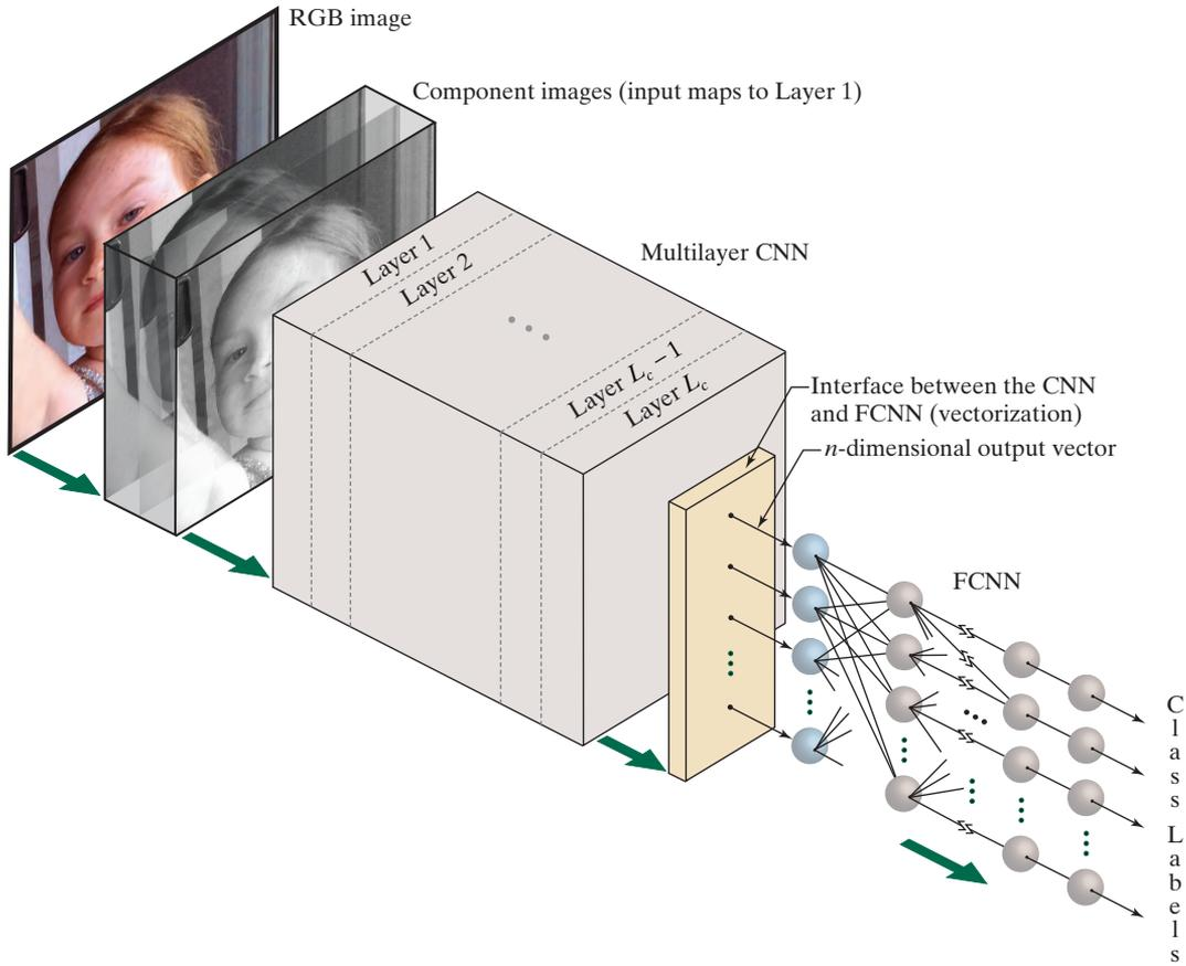
**FIGURE 14.20** General model of the CNN/FCNN architecture we use in this chapter for image classification.
