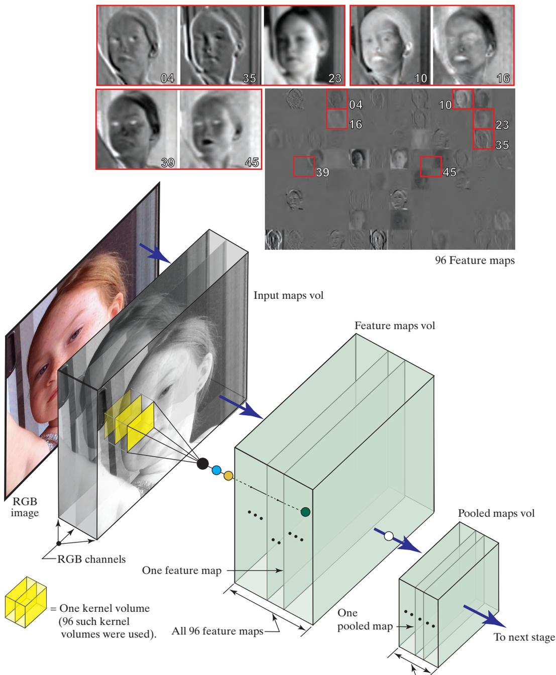
**FIGURE 14.25** Detailed view of the first stage of a CNN, showing the feature maps as images. The highlighted, numbered feature maps shown zoomed at the top, illustrate the types of features extracted by the 96 kernel volumes. The operations performed at the point of the color bullets are explained in Fig. 14.22.
