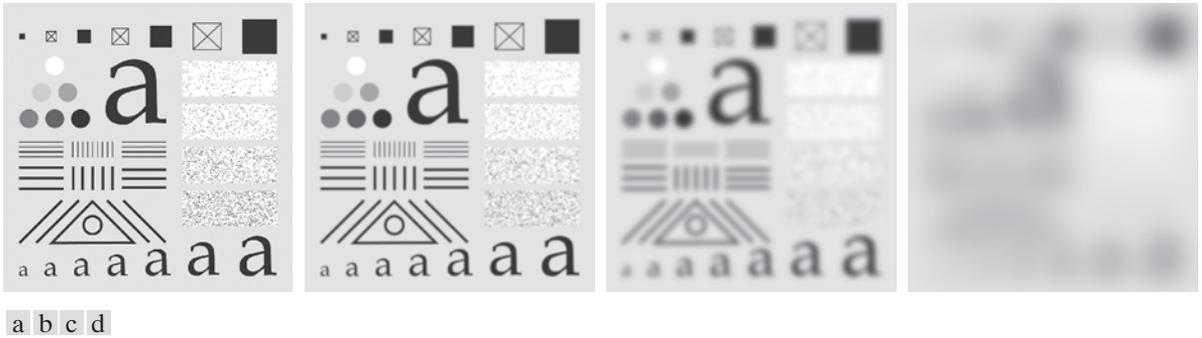
**FIGURE 3.19** (a) Test pattern of size  $1024 \times 1024$  pixels. (b)–(d) Results of using functions `fspecial` and `imfilter` to lowpass filter the image in (a) with Gaussian kernels of various sizes, as explained in the text.
