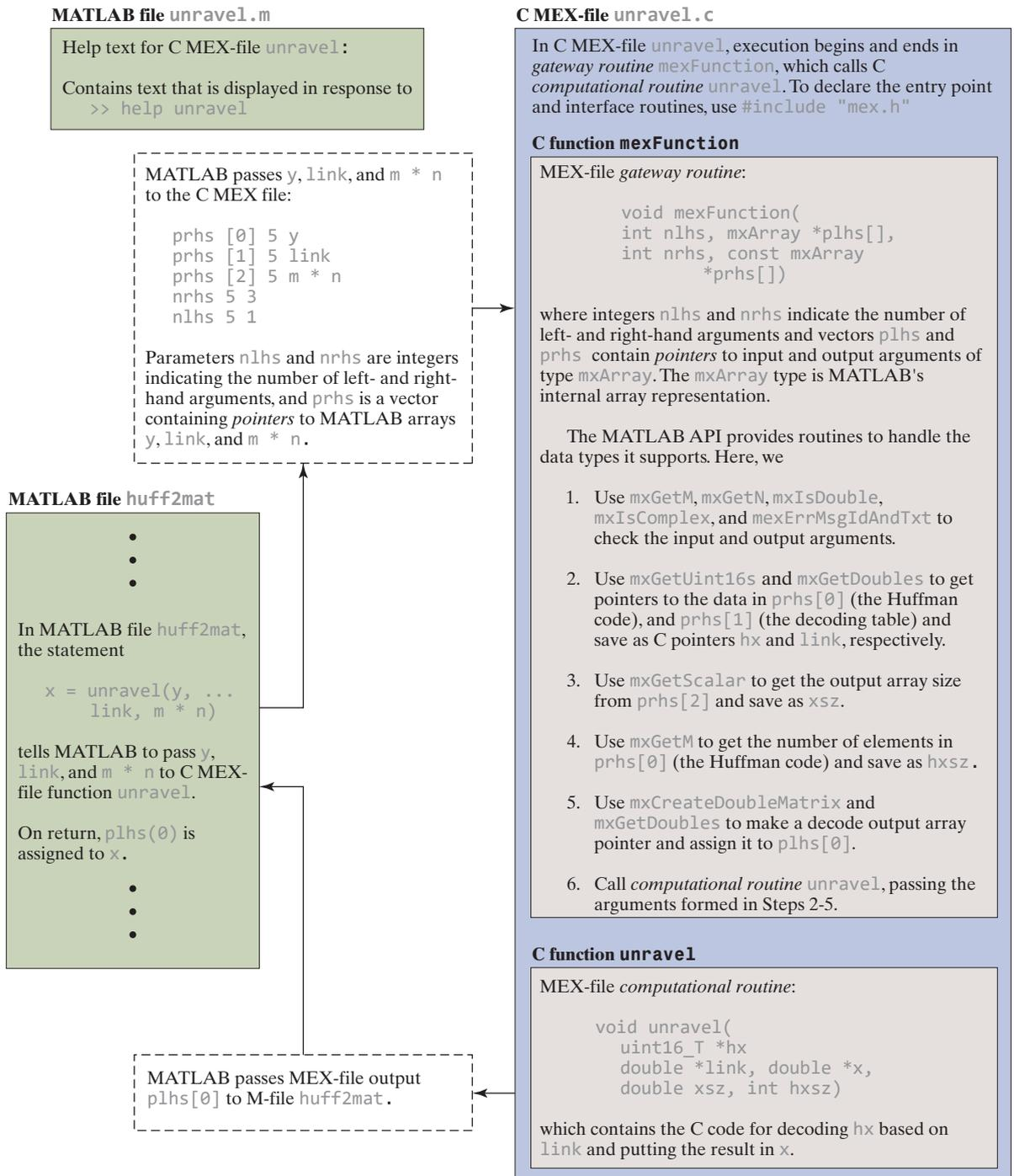
**FIGURE 9.6** The interaction of function `huff2mat` and MATLAB callable C function `unravel`. Note that MEX-file `unravel` contains two functions: gateway routine `mexFunction` and computational routine `unravel`. Help text for MEX-file `unravel` is contained in the separate MATLAB file, also named `unravel`.
