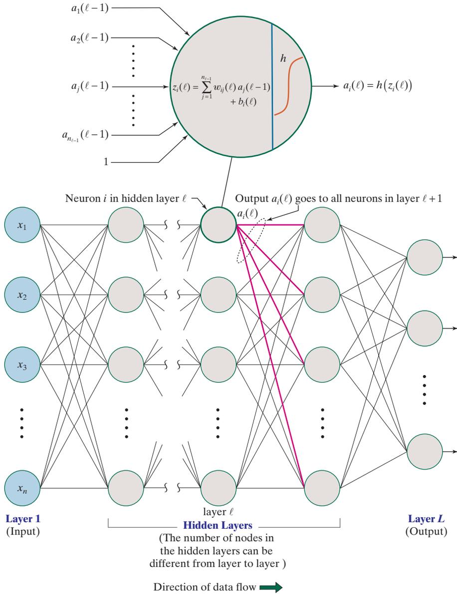
node in the figure, all the nodes in the network are artificial neurons of the form shown in Fig. 14.13, except for the input layer, whose nodes are the components of an input pattern vector  $\mathbf{x}$ . Therefore, the outputs (activation values) of the first layer are the values of the elements of  $\mathbf{x}$ . The outputs of all other nodes are the activation values of neurons in a particular layer. Each layer in the network can have a
